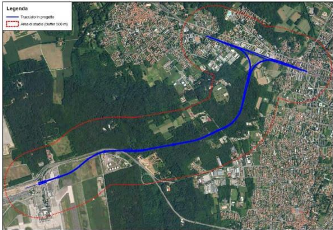
Figure 33: Alignment of the new link T2-Gallarate
